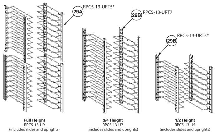
Slides sold in pairs. For additional pair of wire slides, order C5-USLIDEPR-C for Chrome or C5-USLIDEPR-S for Stainless Steel. To order individual universal uprights only, see item #'s 29A, 29B.
