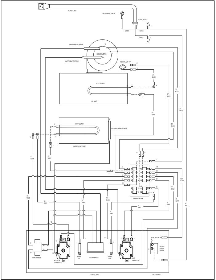
WIRING DIAGRAM — MOISTURE HOLDING MODULE
