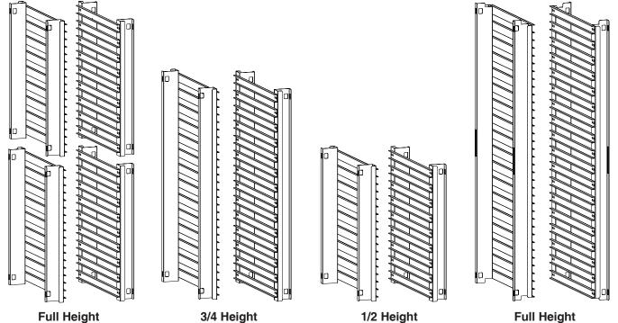
Full Height 2-piece Construction Part No: C5-13-L9D (For Dutch Door Units)
